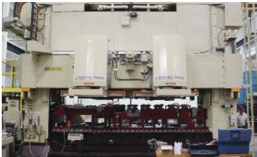
Front-and-back-mounted servo transfer systems feature transfer assemblies placed in the front and back of the press, allowing the press upright window openings to be completely unobstructed, therefore, not limiting the material width of the coil or blank fed in through the window.
