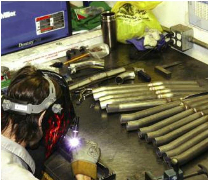
Each fabricated pipe must be identically placed in the fixture in order to perform in exactly the same manner. The high-speed pulsing feature of Big Gun's new welding machine constricts and focuses the arc, allowing operators greater control over arc stability and heat input, allowing parts to stay cool and avoid warping.
