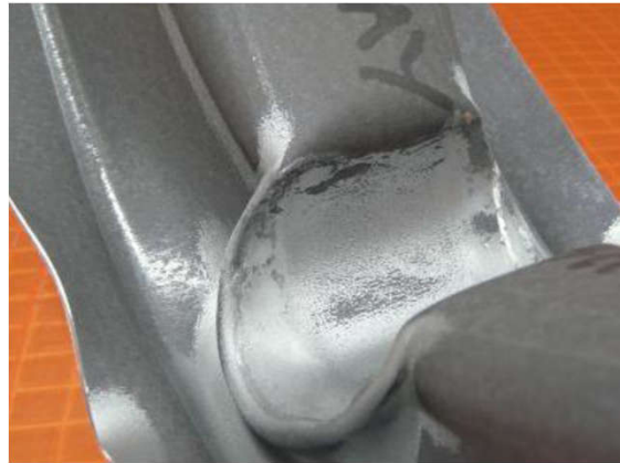
CR1100T-MB @ 120 mm stroke of the crash No crack formation
