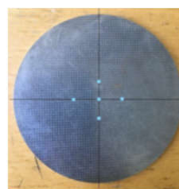
Round blank 7075-T6 2 mm thick 70 mm diameter
