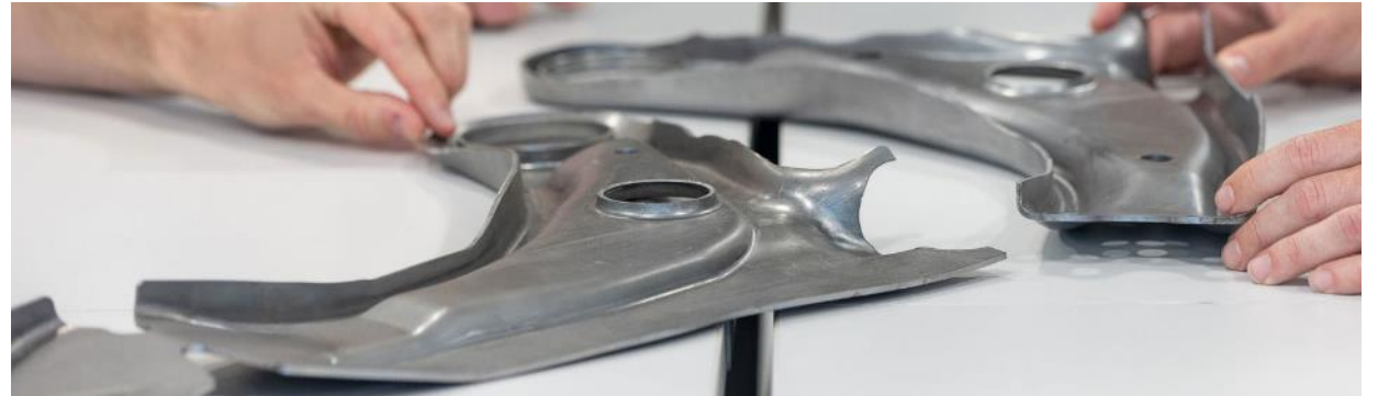
Toyota Yaris Front Lower Control Arm: HR780Y980T-CP
