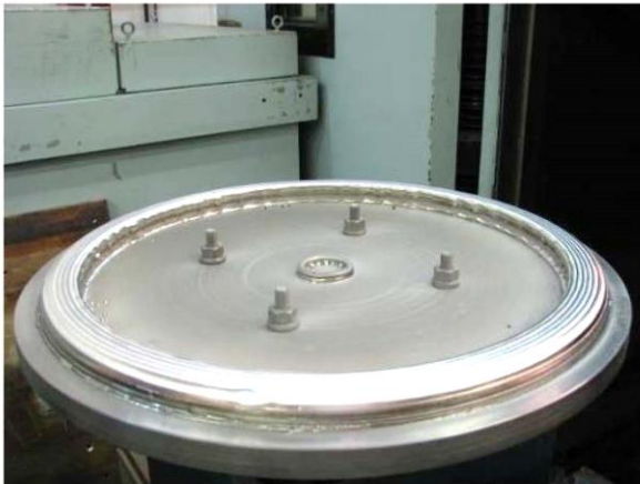
Pictures of the Successive Building of an EB Wire-Feed INCO 718 Deposited Engine Case.
