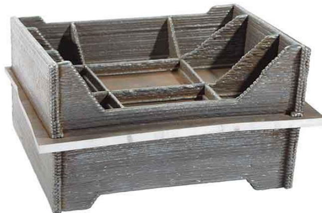
0.6 metre x 0.6 metre titanium frame for BAE Systems http://waamat.com/about/demo-parts
