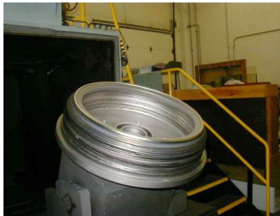
Pictures of the Successive Building of an EB Wire-Feed INCO 718 Deposited Engine Case.
